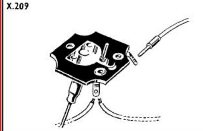
NOTE: To avoid loss of magnetism when withdrawing the armature assembly, a suitable keeper must be applied to the magnet
